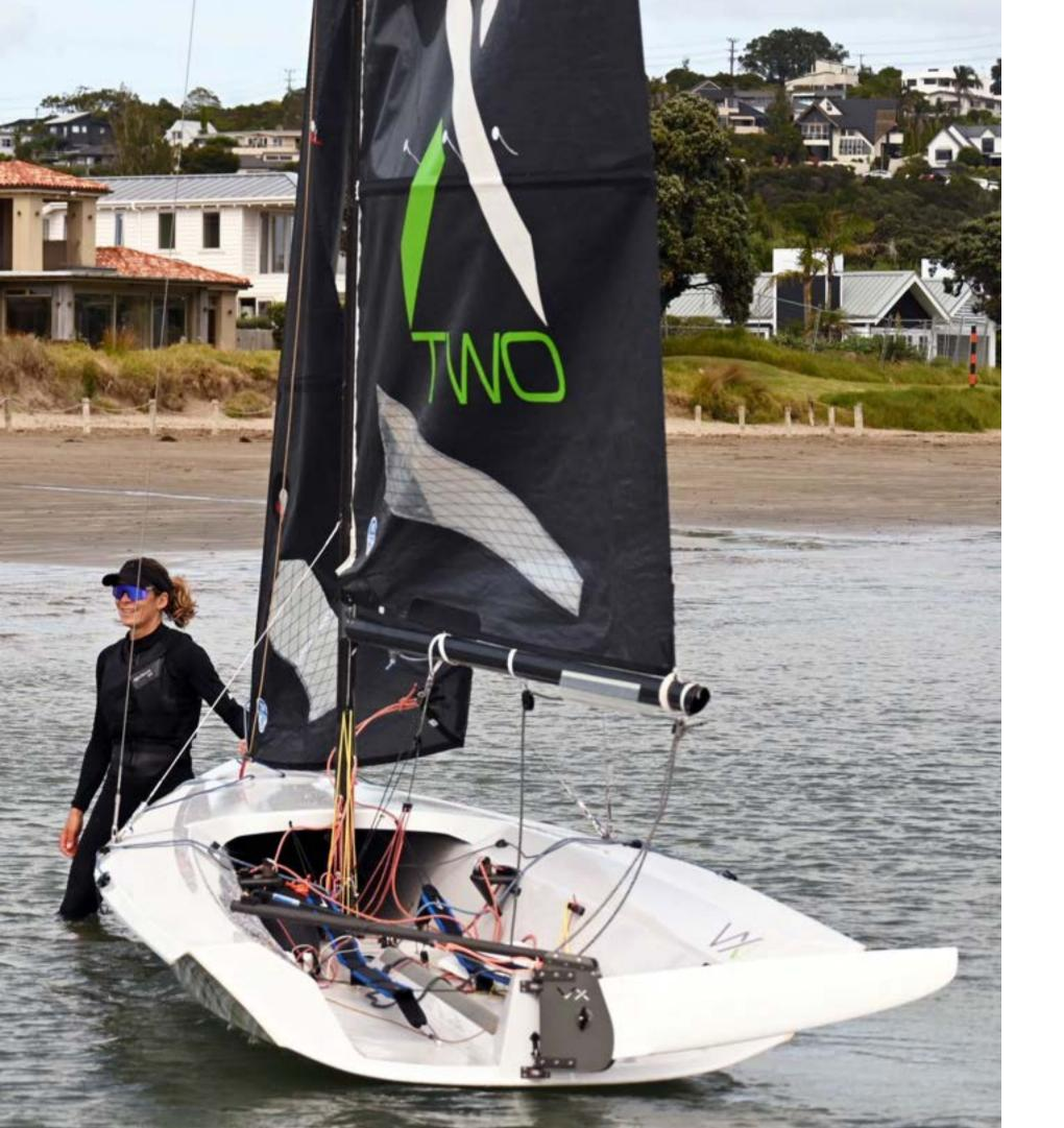
All up weight - 93.24kgs (includes centreboard, rudder stock, tiller, tiller extension, all sails, boom, mainsheet, mast, halyards, stays).
