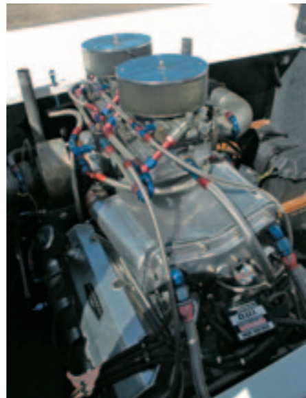
A GALE BANKS TWIN TURBOCHARGED 8.2L CHEVROLET NOW POWERS TOPAZ TO A TOP SPEED OF 80 MPH.
