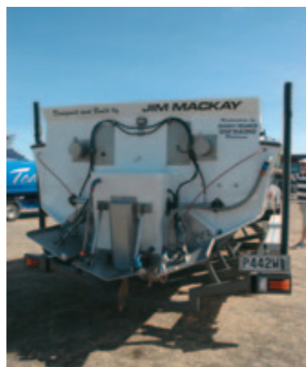
THE TRANSOM AREA HAS BEEN ALTERED WITH A RESHAPED RUDDER AND NEW SHAFT ANGLES.
